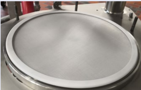
Bottom plate made from stainless steel 1.4404 or Hastelloy® C22 Bodenplatte aus rostfreiem Stahl 1.4404 oder Hastelloy® C22
