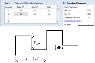
**SWV scan setup and anatomy of the SWV signal** Three parameters define the signal. f, $dE_s$  and  $E_{sw}$  are available on the setup screen.
