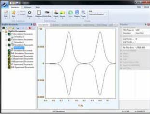
**SVW** simulation and concentration profiles Square waves and concentration profiles can also be simulated with any of the systems described in the CV section. .
