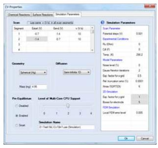
**Setup Screen for the Simulation Parameters** Electrode geometry, dimensionality, pre-equilibria, and a range of computational parameters
