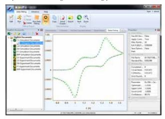
**Data fitting** A group of data files, imported into DigiElch can be fit to a mechanism.
