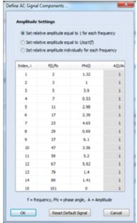
**IMP signal definition** The signal can be defined with up to 15 components with individual frequencies phases and amplitudes. The amplitudes can be fixed to the fundamental amplitude, defined to be  $1/\sqrt{f}$ , or
