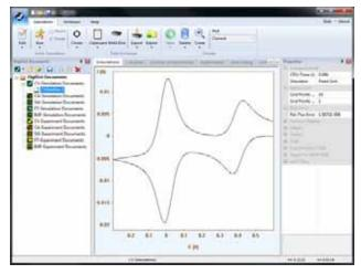
**CV simulations** The simulations can include adsorbed species as well as species diffusing from solution.
