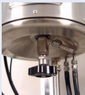
Flush mounted drain valve
