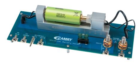
The Universal Battery Holder allows connection of a large variety of batteries, from coin-sized to larger cylindrical shapes (up to 26650), to Gamry Instruments' potentiostats. High currents, up to 30A, may be passed through the battery holder, without danger of destroying the holder. The Universal Battery Holder allows four-point measurements, and is usable with all Gamry Instruments potentiostats, including the 30k Booster.
