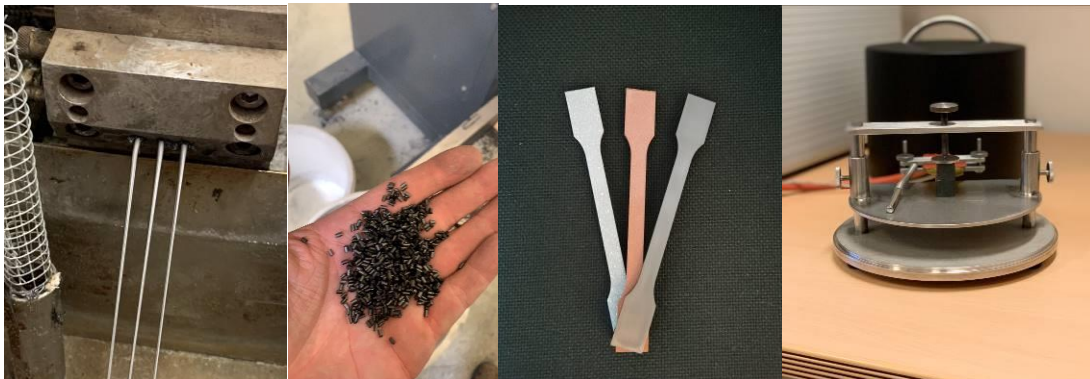
Figure 2: Extruded melt strands (left), granules with graphite (middle left), injection moulded test specimen (middle right), Hot Disk measurement setup (right)
