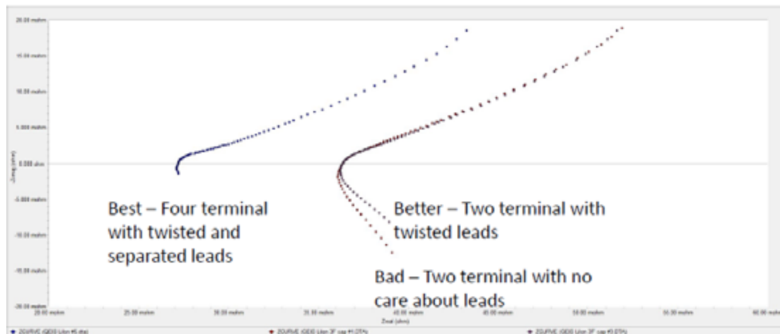
Figure 13: EIS measurement of a 5 F capacitor with 3 different connection schemes.
