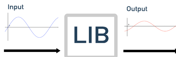
Figure 1. Schematic of EIS on a lithium-ion battery.
