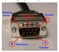
Pins in the Cell Cable for the Series G, PCI4, PC4 Potentiostats, and ECM8 Multiplexer
