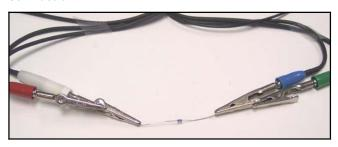
Record the potentiostatic EIS spectrum of this resistor with zero DC and 20 mV $_{rms}$ AC voltage. The frequency range should extend from 0.2 Hz to the system's maximum specified frequency.
