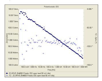
The Bode Plot above is an open lead spectrum measured using a Gamry Reference 600 Potentiostat. Over a wide frequency range, this looks like the spectrum of a small capacitor.
