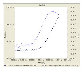
This spectrum fits well to a series RL model with a resistance of 30  $\mu\Omega$  and inductance of 42 nH. The resistance value is interesting. The copper braid used to make the shorted connection has a measured
