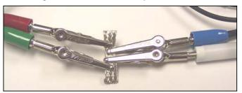
The Working Sense and Reference leads are the inside pair of connections. Don't allow the clip leads to touch except at the braid connections.
