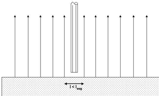
Reduced current density effect -- Current density lines can't adjust to probe
