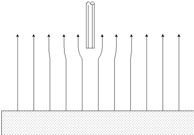
No surface effect -- Current density lines have room to adjust to probe
