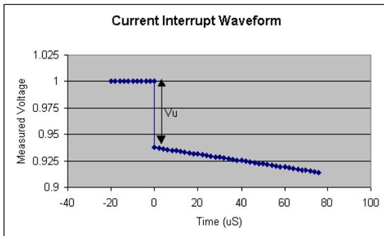
Suppose we are measuring 1.0 V while current is flowing. At time 0 we interrupt the current – very quickly! The voltage immediately drops by the voltage drop across  $R_u$ . Then it starts dropping more slowly.
