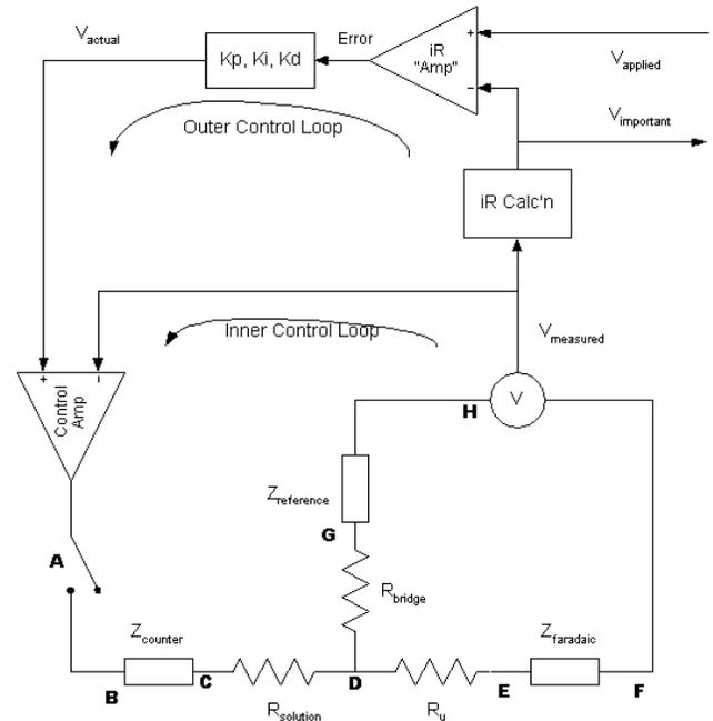
The outer loop does a very similar job to the inner loop but it is implemented digitally in a computer. Its job is to see that  $V_{\text{important}} = V_{\text{applied}}$ , and now the job of the inner loop is to see that  $V_{\text{measured}} = V_{\text{actual}}$ .  $V_{\text{actual}}$  is a new value that comes from the outer loop.
