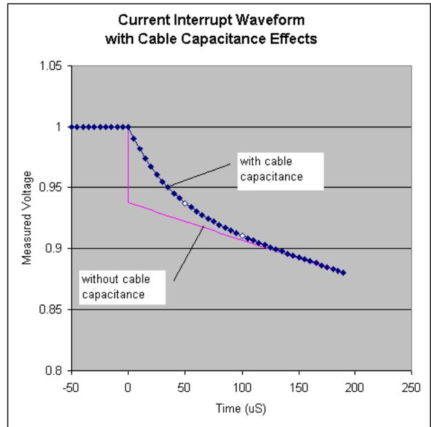
It may be helpful to see this on a log(time) scale so you can see the cell cable & Faradaic capacitors being discharged.
