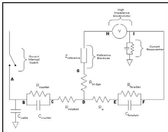
Almost any potentiostat will do a good job of controlling and measuring the voltage between Points H & I.
