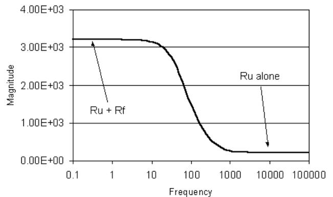
At low frequencies where  $C_f$  is effectively an open circuit, the measured impedance is the sum of  $R_u$  and  $R_f$ . At high frequencies where  $C_f$  is effectively a short circuit, the measured impedance is  $R_u$ .
