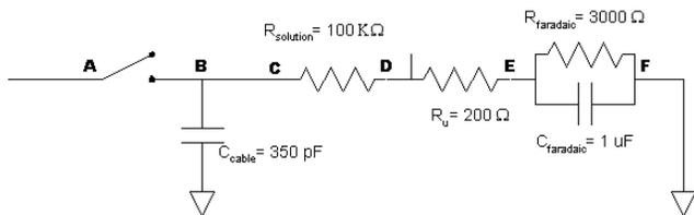
The cable capacitance forms an RC section with  $R_u$  and  $R_{\text{solution}}$ . This means the voltage across  $R_u$  doesn't disappear infinitely fast.
