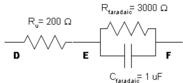
Look at  $R_{faradaic}$ . It has a capacitor,  $C_{faradaic}$  in parallel with it.  $R_u$  doesn't.
