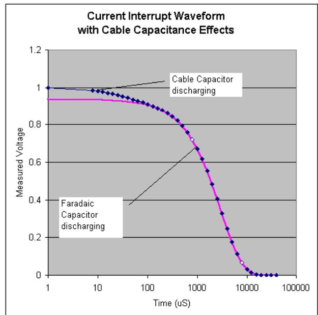
You need to find a time range between the two limiting discharge curves.
