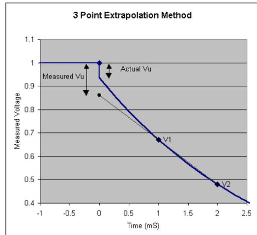
The estimated  $V_u$  is calculated by:  $V_u = V1 + (V1 - V2)$
