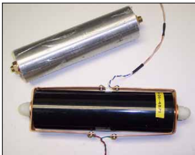
Figure 2 Battery in Fixture and Surrogate
