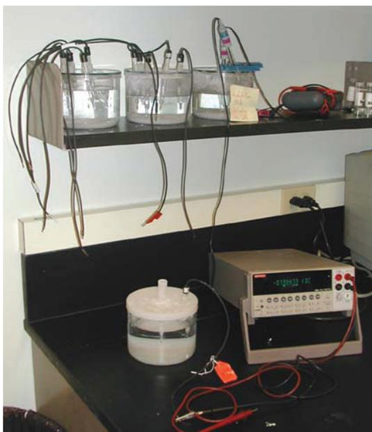
If a Reference Electrode is suspected to be bad, the potential is measured versus the Lab Master. You can do that with a voltmeter, as in the photo, or with your Gamry Potentiostat. If the potential difference is less than 2-3 mV, it's OK. If it's higher than 5 mV, it needs to be refreshed or discarded.
