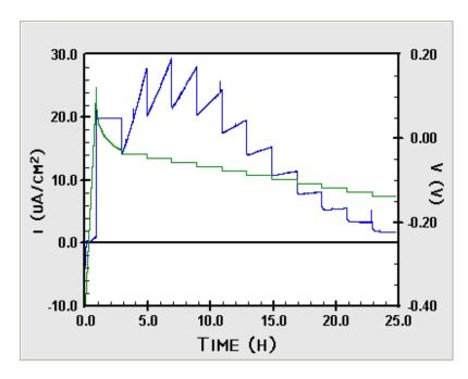
The potential is then stepped towards the original open circuit potential in 10 mV increments. During these potentiostatic steps the current is monitored. If the current continues to increase, that is the indication that crevice corrosion is continuing. If the current does not increase when the potential is held for two hours, then the repassivation potential has been reached.
